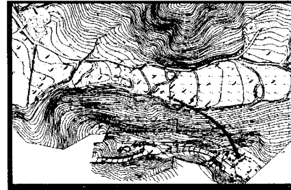
Fig. 47. Groundwater flow direction and particle pathlines(MODPATH)
