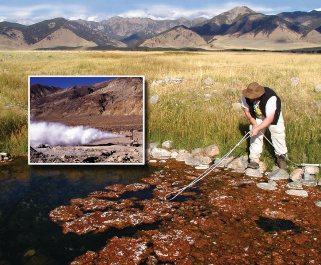
Sampling a warm spring in northern Nevada for gas and isotope analysis as part of a geochemical survey of the northern Basin and Range. Inset shows a geothermal well under test at the Dixie Valley geothermal field.
